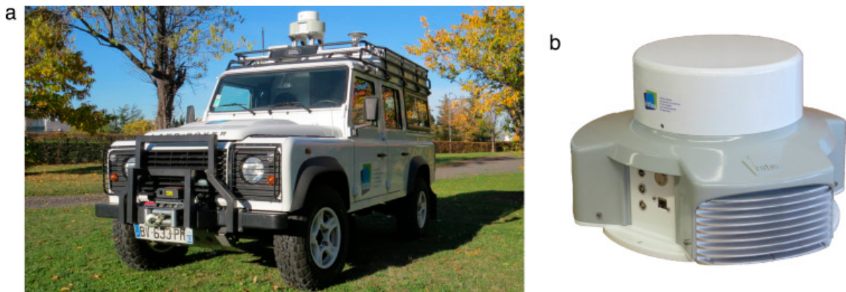
Figure 3: PELICAN radar (a) positioned on an experimental vehicle, and (b) detailed view [26].
